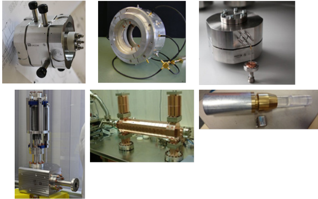
Fig.9: Upper row: Beam Position Monitor, Charge monitor, dark current monitor. Lower row: Screen monitor, transverse deflecting rf structure, beam loss monitor
