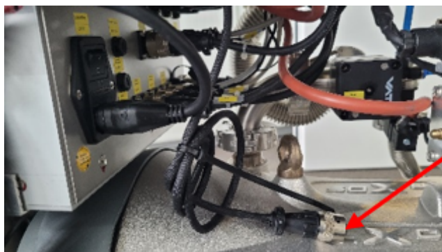
Heating connector to connect with the heating controller
